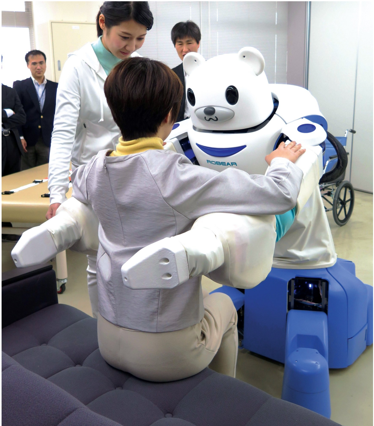
Japan is a pioneer in care automation. Well-known devices include this prototype lifting robot, Robear.
